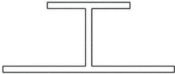
**PJ 2 Top & Bottom Runner Rail & End Cap** - used to finish ends as a top & bottom track cut edges top & bottom as well as the end of a straight run
